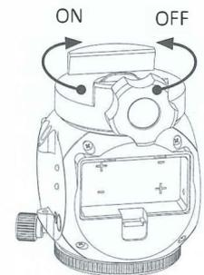
SAM will rotate left to right if **Clockwise** is set to **ON**, or right to left if **Clockwise** is set to **OFF**.
