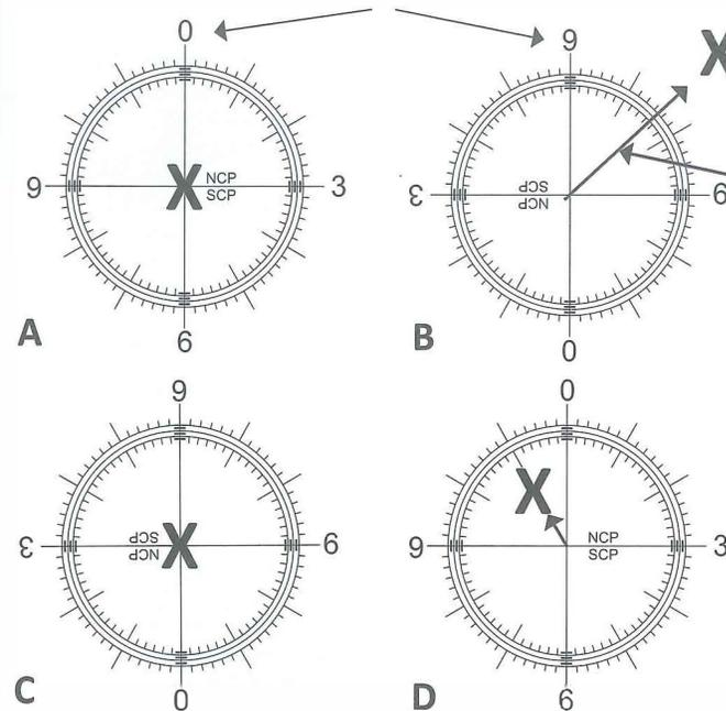
These figures represent the view through the polar scope when a target is initially centered (A), after Polar Scope has been rotated 180 degrees (B), after the reticule adjustment has been made and SAM has been re-centered on the target (C), and the target displacement after the second 180 degree rotation. There is a bit of displacement left as shown here, but one more iteration of the reticule alignment is likely all that would be needed to remove it.
