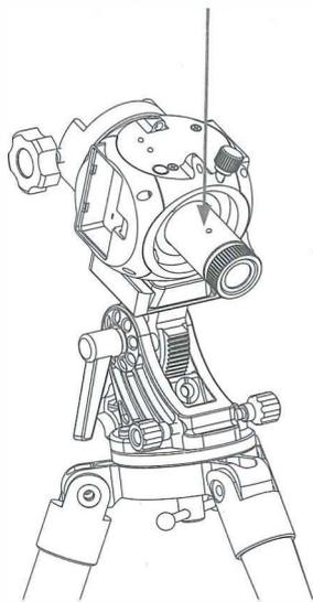
**CAUTION: DO NOT over tighten the screws as you may crack the glass reticule inside the eyepiece of the polar scope.**
